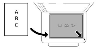
**Note:** If you are using Epson ScanSmart to scan multiple photos at once, just make sure they are at least 0.2 inch (4.5 mm) away from the edge of the scanner glass and at least 0.8 inch (20 mm) away from each other.
