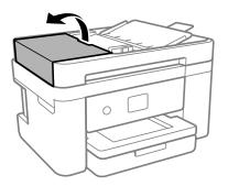
4. Carefully remove any jammed pages from beneath the ADF.
