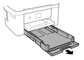
3. Squeeze the tab on the right edge guide and slide the edge guides outward.
