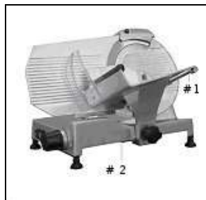
Figure 10 – Lubricating the sliding rods
