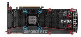
For RTX 3090 XC3 ULTRA and XC3 cards: Removing the backplate may require some force to loosen up the thermal pads. Make sure to place the thermal pads on the backplate as shown in the image below, as you will reuse the backplate and thermal pads.
