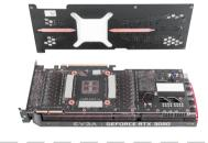
2. Turn the card over and remove the heatsink from the card. Remove the fan connectors (blue, beige, and black) first, and then the LED connector (black) as you lift the heatsink off the card.
