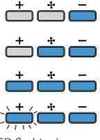
Speed 1<br>Speed 2<br>Speed 3<br>Speed 4<br>("+" LED flashing) |
