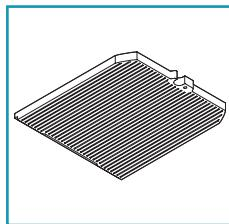
Active carbon filters have the function of retaining odours in the air flow passing through them. The air, purified by running many times through the filter, is recirculated into the kitchen. Active carbon filters **cannot be washed** and are to be immediately replaced every **3-4 months** (depending on the frequency of use of the hood). Dispose of the active carbon filters in compliance with the regulations in force in the country of use.
