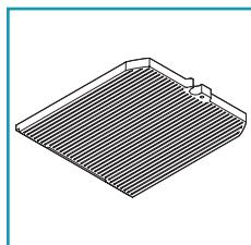
Active carbon filters have the function of retaining odours in the air flow passing through them. The air, purified by running many times through the filter, is recirculated into the kitchen. Active carbon filters **cannot be washed** and are to be immediately replaced every **3-4 months** (depending on the frequency of use of the hood).
