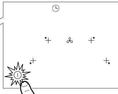
Press and hold the On/Off button (1) for 2 seconds to turn the hob on and activate its functions. All the Digits show *B*, and the Timer digits show "C L".
