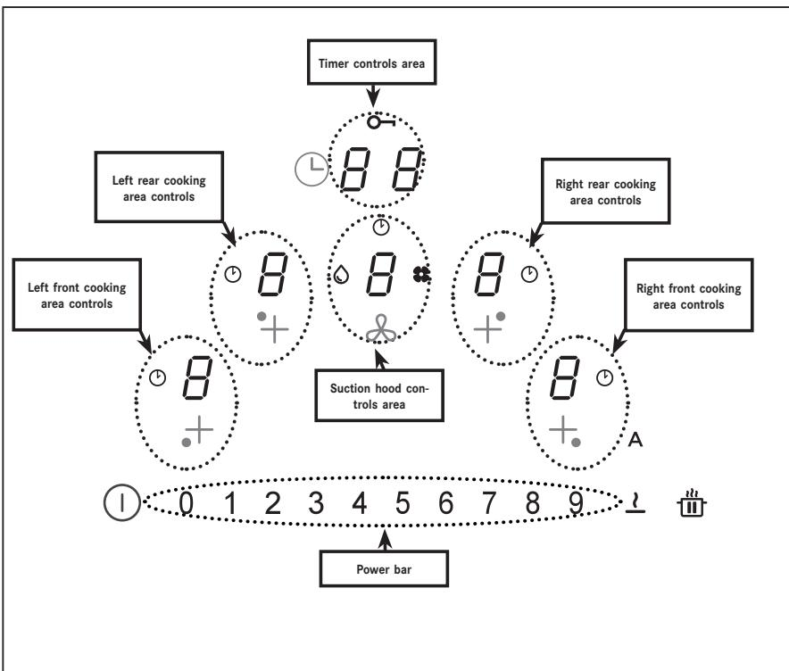
The controls for the cooking areas, suction hood and timer can be activated by pressing on the reference Digit 8.
