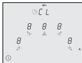
At this point the hob is on but all the cooking areas and the hood are at zero power. The Hob will switch off automatically after 20 seconds if it is not used.
