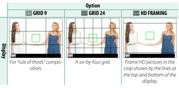
Framing guides are not shown at default settings but can be displayed using **Z** SCREEN SET-UP > DISP. CUSTOM SETTING (■ 19).
