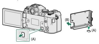
**3** Place the fan on the camera, making sure the screws and connectors are correctly aligned.
