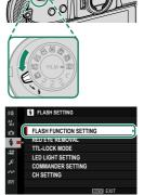
Sync terminal options will be displayed if the built-in flash is lowered and either no flash unit, or an incompatible flash unit, is mounted on the hot shoe (I 359). Raise the flash before adjusting settings. 3 Highlight items using the focus stick (focus lever) and rotate the rear command dial to change the highlighted setting (III 121).
