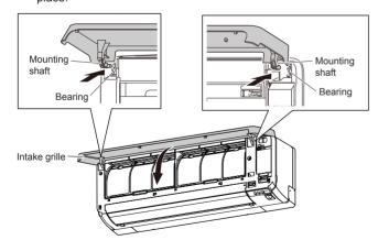
Press 4 places on the intake grille to close it completely.
