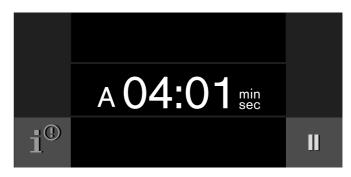
For some dishes, during the preparation stage, the display shows information about turning or stirring. Follow this information. When you open the appliance door, the operation stops. After the door is closed, continue the operation by touching •. If you do not turn or stir the food, the programme will continue on until its end, as normal, anyway.
