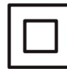
This appliance has been designed with a double-insulation system for your safety. **CE**
