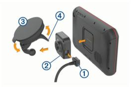
2 Press the mount ② onto the suction cup ③ until it snaps into place.
