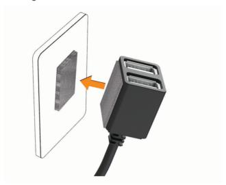
8 Connect the USB power cable from your Garmin Dash Cam device to a USB port on the Constant Power Cable device.
