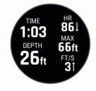
In-dive screen: Displays the information about the current dive, including the elapsed time, current and maximum depth, heart rate data, and rate ascent or descent.
