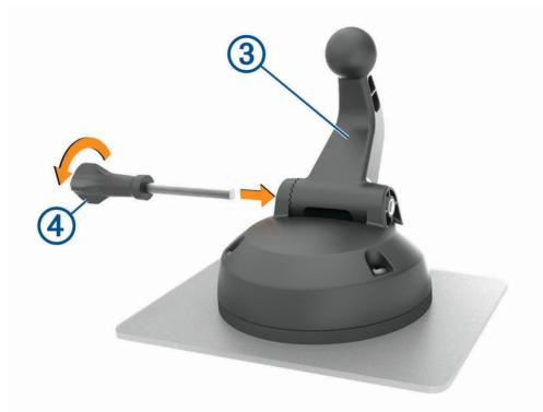
6 Insert the thumbscrew ④ into the mount and tighten it to secure the ball mount arm.
