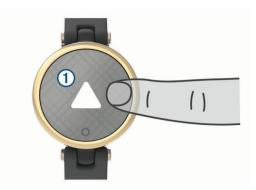
2 To turn the screen off, rotate your wrist away from your body. NOTE: The screen turns off when not in use. When the screen is off, the device is still active and recording data.
