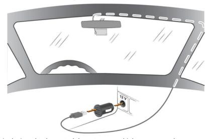
The shorter cable is designed to be routed down to your vehicle power supply.
