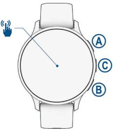
(A) Action button: Hold for 2 seconds to turn on the watch.
