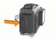
2 While pressing the release latch, pull open the front of the latch ②.
