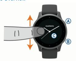
(A) Action button: Press to turn on the device.
