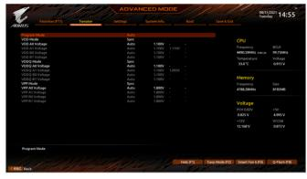
These items allow you to adjust DDR5 memory voltages. This submenu is only present on models that support DDR5 memory.
