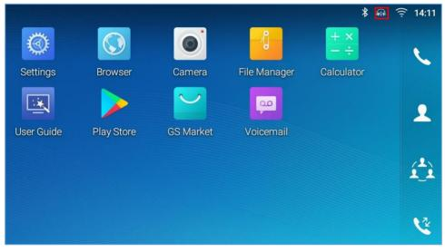
Figure 153: USB Headset Connected
