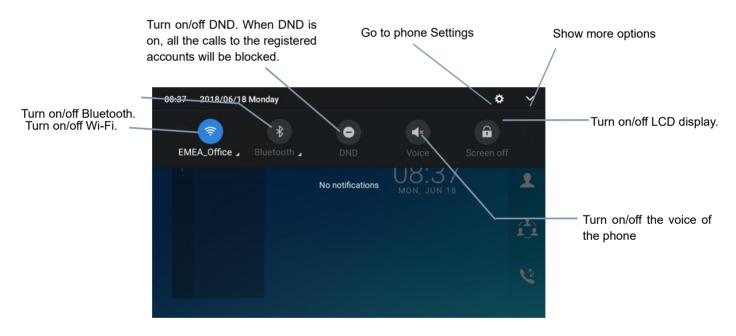
Figure 27: System Settings in Status Bar
