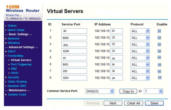
Figure 2-13 Port Mapping on Router
