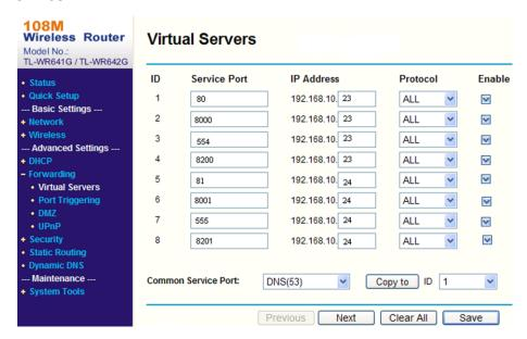
Figure 7-1 Port Mapping on Router
