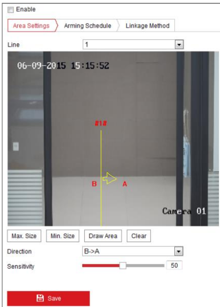
Figure 10-21 Line Crossing Detection
