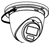
Figure 2-46 Snap the Camera into the Gang Box
