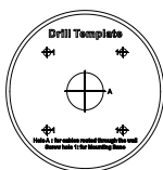
Figure 2-12 Drill Template of the Junction Box
