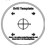
Figure 2-15 Drill Template of the Junction Box
