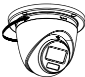
Figure 2-46 Snap the Camera into the Gang Box
