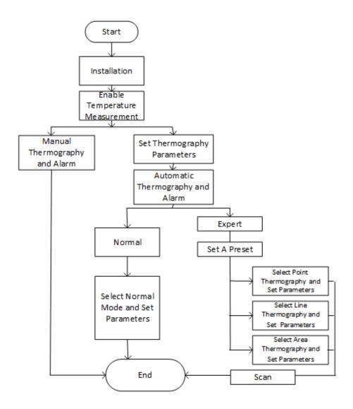
Figure 3-1 Thermography Configuration Flow Chart
