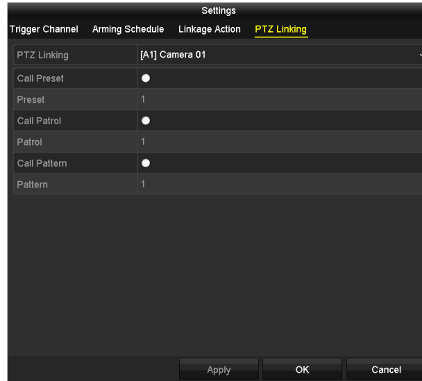
Figure 8-8 Set PTZ Linking of Alarm Input
