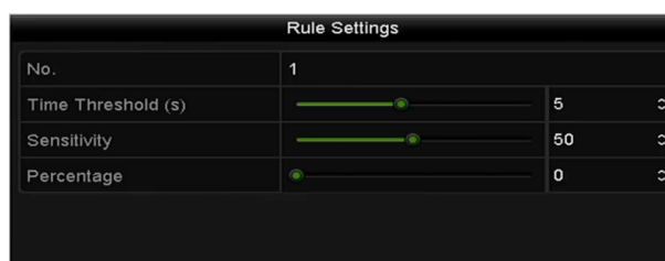
Figure 10-7 Set Intrusion Crossing Detection Rules
