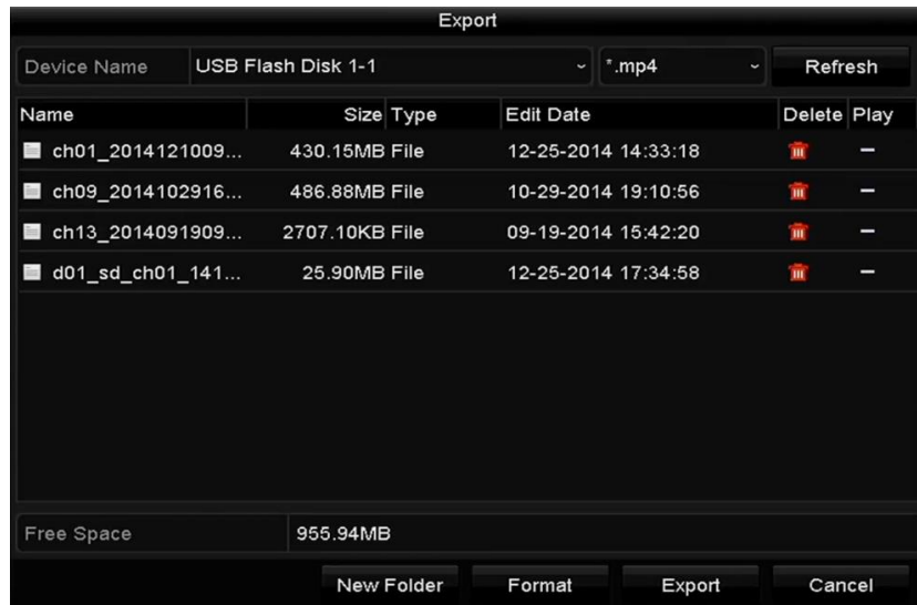
Figure 7-12 Storage Device Management
