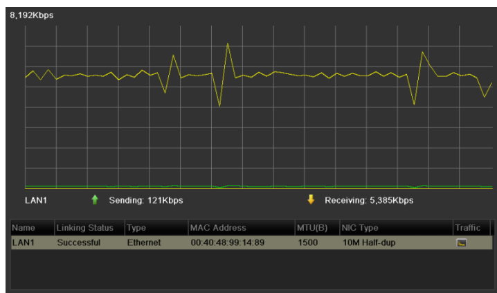
Figure 12-25 Network Traffic Interface
