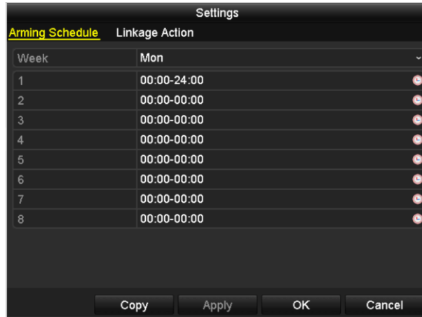
Figure 8-12 Set Arming Schedule of Video Tampering
