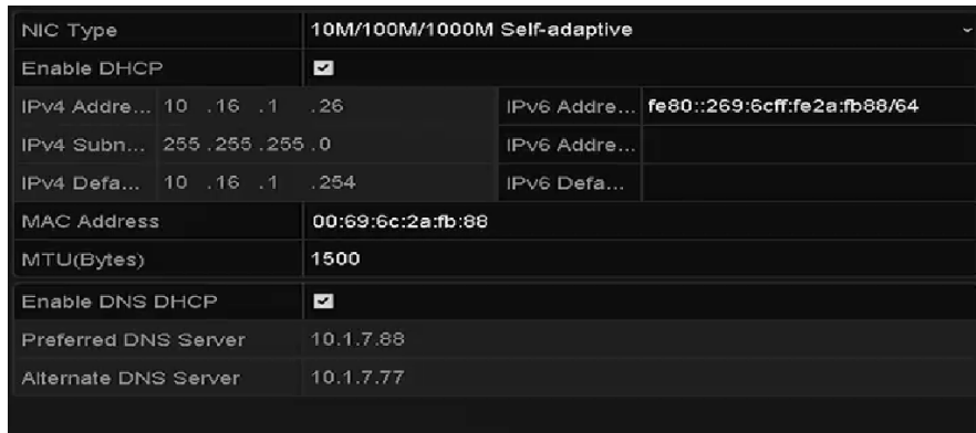
Figure 12-16 Network Settings Interface
