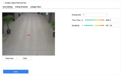
**Figure 5-9 Object Removal Detection**
