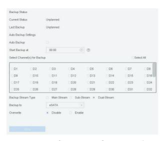
Figure 8-5 Configure eSATA for Auto Backup
