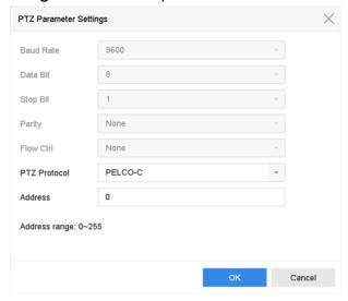
**Figure 3-10 PTZ Parameters Settings**
