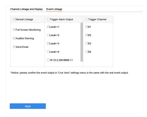
**Figure 9-6 Set Trigger Cameras of POS**
