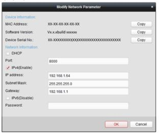
**Figure 1-6 Modify Network Parameters**
