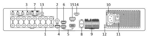
Figure 1-16 Rear Panel of DS-7300HUHI-K4 (with 16 Video Inputs)
