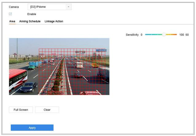
Figure 11-3 Set Motion Detection
