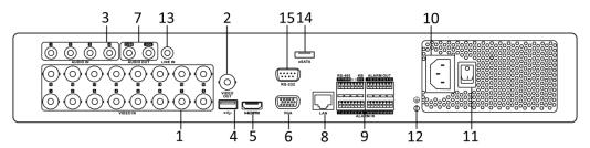
Figure 1-15 Rear Panel of DS-7300HQHI-K (with 16 Video Inputs)
