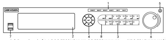
Figure 1-2 Front Panel of 1.1.2 DS-7300HQHI-K4, DS-7300HUHI-K4, and iDS-7316HUHI-K4/16S
