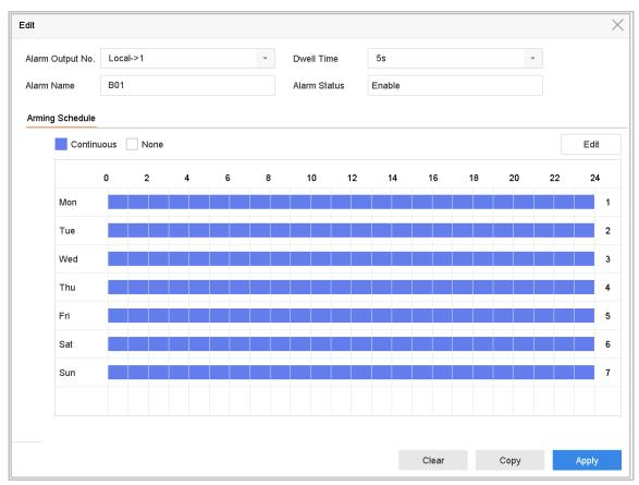
Figure 11-8 Alarm Output
