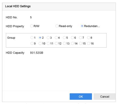
Figure 7-12 HDD Property-Redundancy
