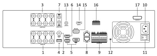
Figure 1-17 Rear Panel of DS-9000HUHI-K8 (with 8 Video Inputs)
