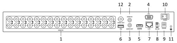
Figure 1-13 Rear Panel of DS-7200HQHI-K (with 32 Video Inputs)
