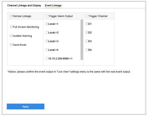
Figure 12-8 Set Trigger Cameras of POS
