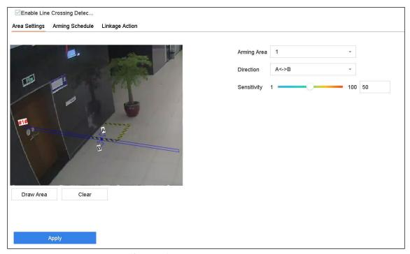
Figure 13-4 Line Crossing Detection
