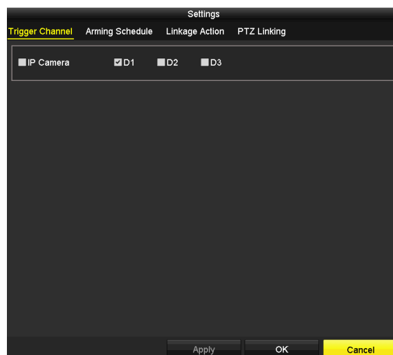
Figure 5-17 Set Trigger Camera of VCA Alarm
