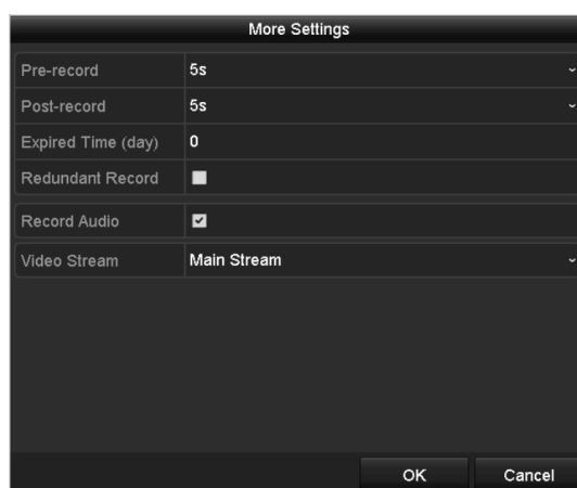
Figure 5-3 Recording Parameters-More Settings
