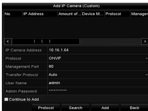
Figure 2-24 Custom Adding IP Camera Interface
