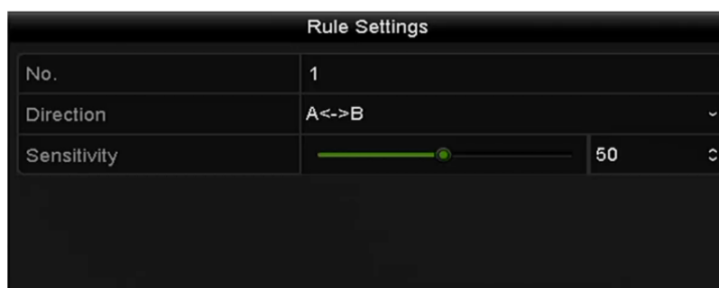
Figure 8-13 Set Line Crossing Detection Rules
