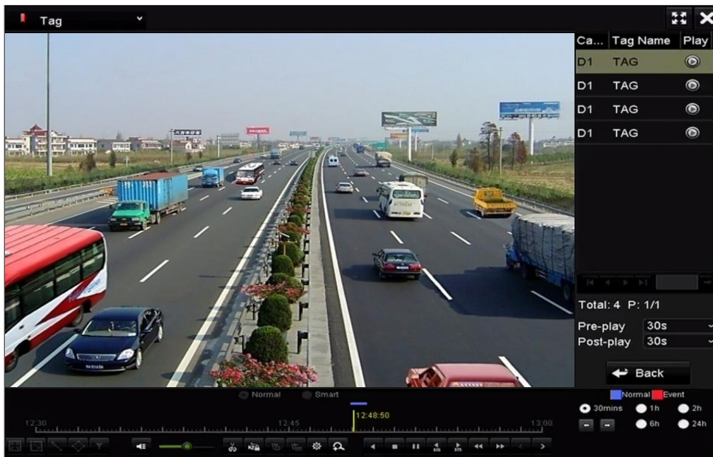
Figure 6-14 Interface of Playback by Tag
