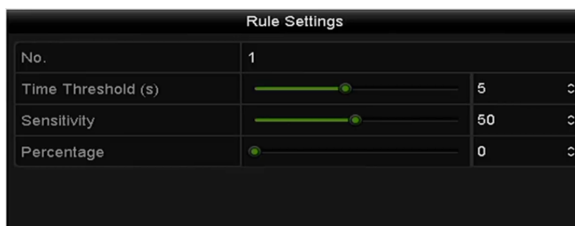
Figure 8-15 Set Intrusion Crossing Detection Rules
