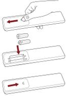
1. Slide the back cover to open the battery compartment of the remote control.
