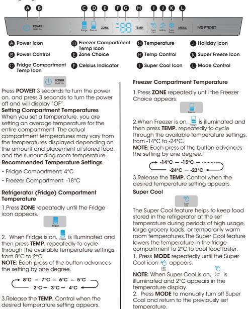
**NOTE:** Super Cool will automatically turn off after 3 hours, and the refrigerator will revert to its previous temperature setting.
