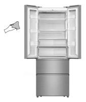
Although this appliance automatically defrosts, a layer of frost may occur on the freezer compartment's interior walls if the freezer door is opened frequently or kept open too long. If the frost is too thick, choose a time when the freezer is nearly empty and proceed as follow:
