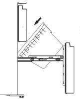
2. Put the tray on the drawer and push it award and ensure the tray's rollers on the freezer liner (D)'s fillets.
