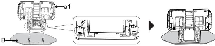
5. Secure the two M4×8 screws to screw holes on the back of TV as the illustration shows.
