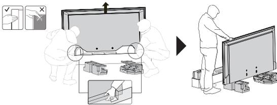
3. Take out the base stand Part A and open it from top, then separate it into Part a1 and Part a2. And you will find two M4x8 screws.
