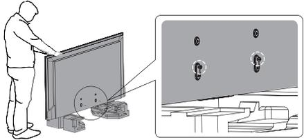
6. Hang the assembled Part a1 and Part B to the two M4×8 screws you have secured to the TV, then secure the assembled part to TV with four M5×16 screws. You can adjust the height of base stand to H1 or H2. For H1, secure screws to four hole 1. For H2, secure screws to four hole 2.
