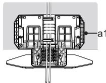
8. Place Part a2 on Part a1 and assemble them together. Then tap the four sides of the Part a2.
