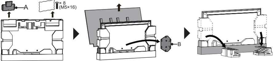
2. Two people stand on each side of the TV. Hold the side of the TV with one hand and hold the bottom with the other hand. Lift and move the TV vertically to the side cushions. Do not pinch the screen when hold the TV.
