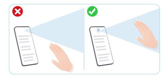
3 To scroll up, hold the back of your hand towards the screen with your fingers closed together and extended, and then wave your hand up when icon stably appears on the screen.
