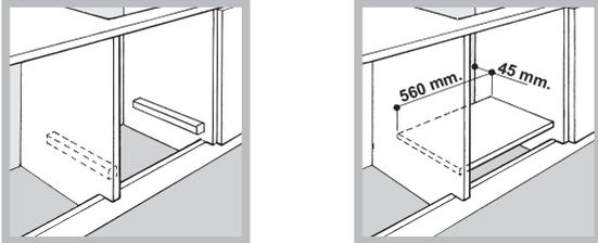
Where a hob is installed above an oven without a forced ventilation cooling system, adequate ventilation must be provided inside the cabinet by means of air holes through which air can pass (see figure).
