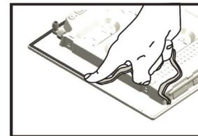
Apply the seals that come with the appliance along the outer edges of the hob to prevent any passage of air, humidity and water (see Figure).
