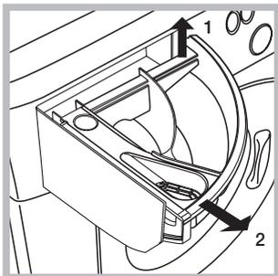
Remove the dispenser by raising it and pulling it out (see figure). Wash it under running water; this operation should be repeated frequently.
