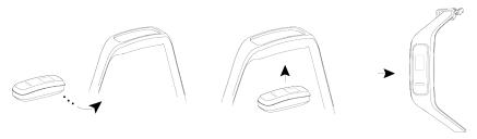
2. The band strap adopts a U-shaped buckle designs. To wear the band, insert one end of the strap through the U-shaped buckle and then fasten it.
