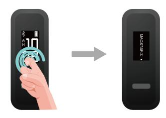
**Method 2:** View the Bluetooth name and MAC address on the back of your band body. The Bluetooth name of your band is **HUAWEI Band 3e-XXX**, while the band's MAC address is in 12 alphanumeric characters next to **MAC:** .
