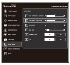
Press the ENTER Button and finally the EXIT Button to close the On Screen Display feature. All changes are saved in the memory.
