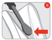
Immerse the steam arm in the milk 5, turn the steam knob counterclockwise and wait for the milk to froth
