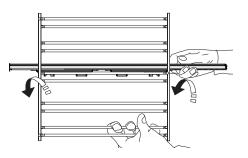
**4.** To secure the guide, press the lower portion of the clip firmly against the shelf guide. Make sure that the runners can move freely.
