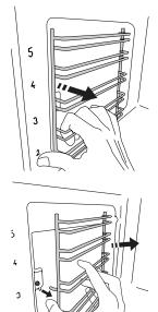
• **To reposition the shelf guides**, position them near the cavity and initially insert the two pins into their lodgings. Next, position the external part near its lodging, insert the support, and firmly press towards the wall of the cavity to make sure the shelf guide is properly secured.
