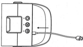
3.Pressing the power switch, the unit will start to work in Gear I and the power red light will be flashing. Pressing the power switch again, the unite into Gear II and the power light will change green. Pressing it for the third time, the wind speed is Gear III and the light will change Blue. When the button is pressed again or long pressed in any state, the unit shuts down (From I>2>3>Close)
