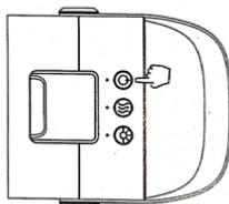
4.Mist function can be used separately, or worked together with the fan.
