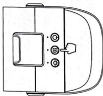
Note: Please make sure that there is water in the water tank when you press "Mist" button. When there is no water in the water tank, please pay attention to add the water or stop the humidification function in time, otherwise the unit will be damaged.
