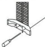
Before using the product, assemble the base (supplied in the carton). To do this, use the 4 self-tapping screws supplied, taking care to set them correctly in the lower ends of the side of the device.
